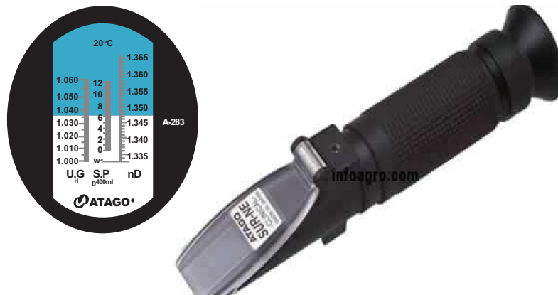
Fig. (2). Refractometer and scale used to measure IgT in blood serum.
