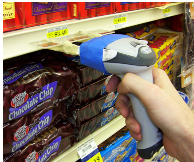
Fig. (6). The barcode scanner, with the added stabilizers, resting on a shelf lip.
