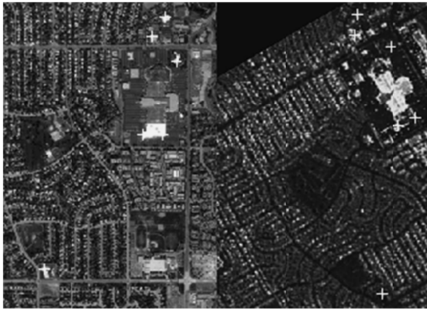
Fig. (3). Final set of detected control points (as indicated by crosses). (Left) Optical image. (Right) LiDAR image. Note: This Figure shows the effectiveness of the methodology developed by Wong and Orchard [13] in control point detection. Courtesy: (Wong and Orchard 2008), IEEE transactions on Geoscience and Remote Sensing.
