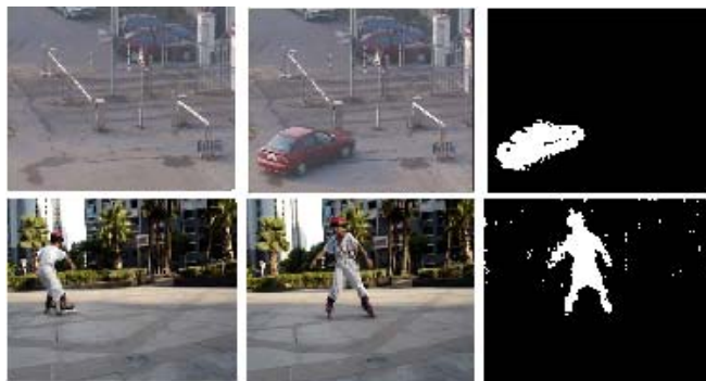
Fig. (4). Outdoor detected foregrounds. The first column is the first frame of their corresponding sequences, the second column is the current frame (60#, 115# from top to bottom, respectively), and the third column is the detected foreground.
