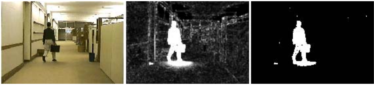
Fig. (1). Detection using value component of HSV for Hall Monitor (frame #47). Original image, E_{\Delta V} image, and extracted possible moving object regions from left to right, respectively.
