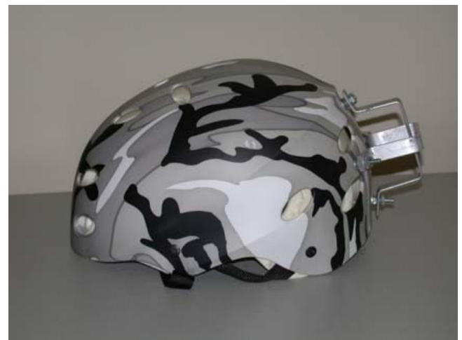
Fig. (1). (a) skier vest with accelerometer 'pocket' located on left anterolateral aspect of the torso, (b) Skier helmet with accelerometer mounting frame on the posterior aspect.
